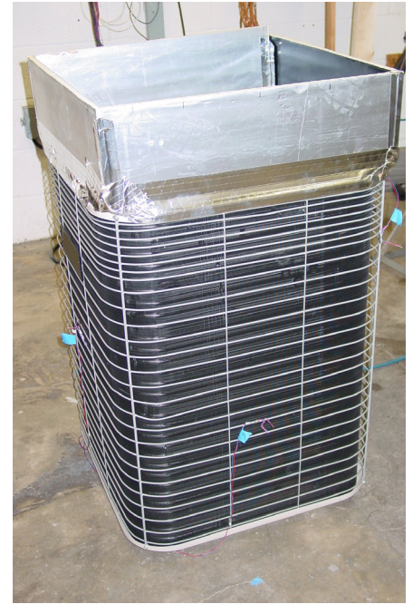
Figure 2. ASHP test unit in chamber – outdoor section
