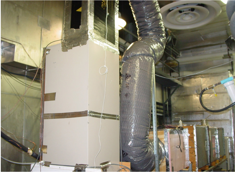
Figure 1. ASHP test unit in chamber – indoor section
